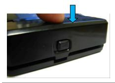
As indicated in the illustration, close battery compartment cover and press on it until latches into the base part.
