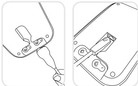
Connect your charging station to the mains and to the local area network with the provided network cable and power adapter.
