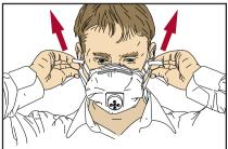
**5** Check the straps are not twisted. If you need to tighten the straps, pull both ends at the same time, bottom first, then top.
