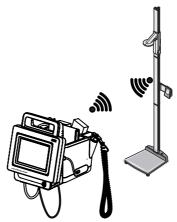
In order to be able to communicate with devices from the **seca 360° wireless** system, the **seca 360° wireless** module of the mVSA/mBCA must be activated and a wireless group set up.
