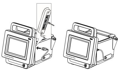
Connect the USB cable of the SmartBucket to a free USB port of the monitor.
