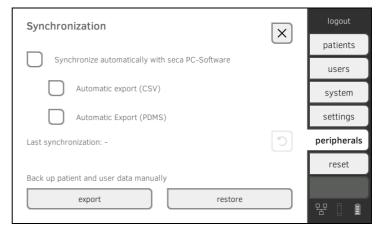
3. Press the **Synchronize automatically with seca PC software** checkbox.
