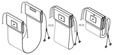
2. Suspend the measuring mat in the magnetic catch as shown in the illustration below.
