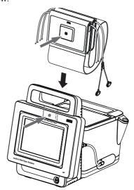
3. Ensure that the measuring mat is correctly located in the magnetic catch of the monitor.
