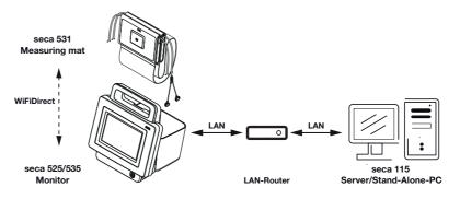
If you connect the device to your network via LAN cable, the measuring mat, if present, can communicate with the monitor via the factory-activated **WiFi direct** connection. This allows data to be exchanged even when the measuring mat is not hung in the magnetic catch of the monitor.
