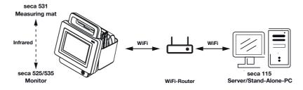
If you connect the device to your network as a WiFi client, the measuring mat, if present, can only communicate with the monitor via the infrared interface.
