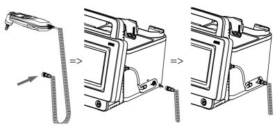
Put the connector for the in-ear thermometer in the socket on the Smart-Bucket until you feel the connector engage.
