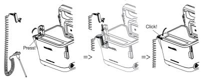
4. Push the temperature probe completely into the probe holder as shown in the illustration below.
