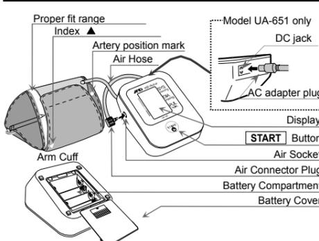
Note: Model UA-611 doesn't have the DC jack for AC adapter. The DC jack is located on the rear of the model UA-651 only. The AC adapter is an optional accessory (sold separately)
